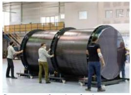
Spectrum manufacturing of main stage structural segments at Isar Aerospace company premises in Ottobrunn, Bavaria. [3]
